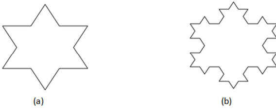
Figure 2. The Koch Snowflake antenna: a) First iteration, b) Second iteration.
