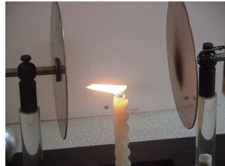
Figure 4. Candle flame under the influence of a left-directed electric field: the upper part of the flame, which is positively charged, deviates to the left, and the lower part of the flame, which is negatively charged, deviates to the right [12].
