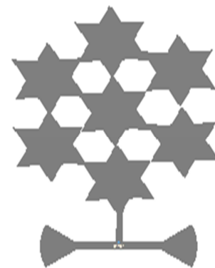
Figure 4. Design of Koch fractal with bowtie antenna.
