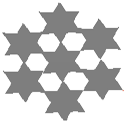
Figure 3. Design of Koch fractal antennas.
