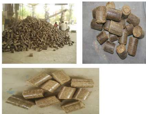
Fig. 2.1. Different crop residue briquette produces at energy enclave CIAE, Bhopal
