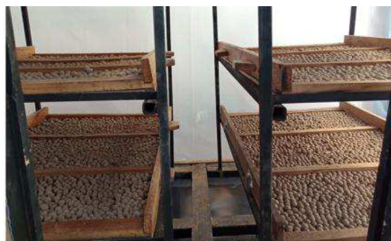
Figure 10. Loaded Solid Clay- \text{CaCl}_2 desiccants in the greenhouse desiccant.
