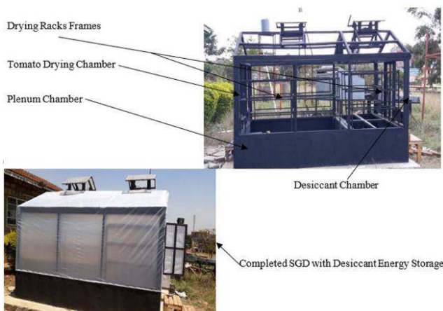
Figure 2. Constructed SGD with Solid \text{CaCl}_2 - Clay Desiccant energy storage system Photo.
