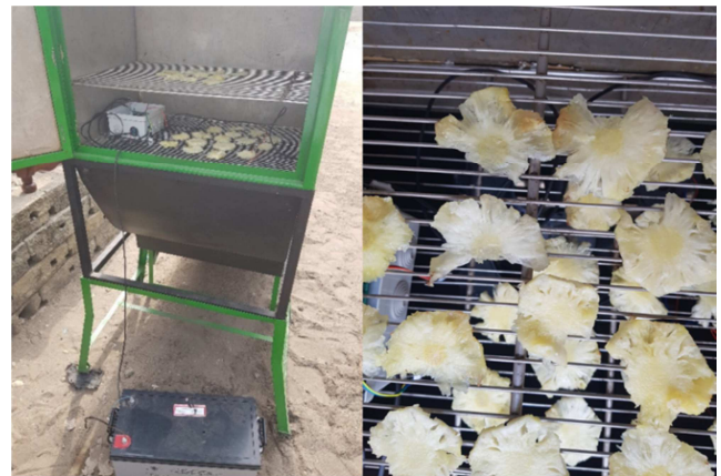
Figure 7. Arrangement of pineapple slices in the drying chamber.
