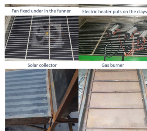
Figure 9. Some details about the solar dryer.
