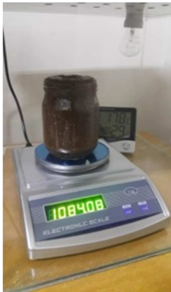
Figure 4. Actual Experimental Setup for the Evaporation Test for the Brown Clay Sample.
