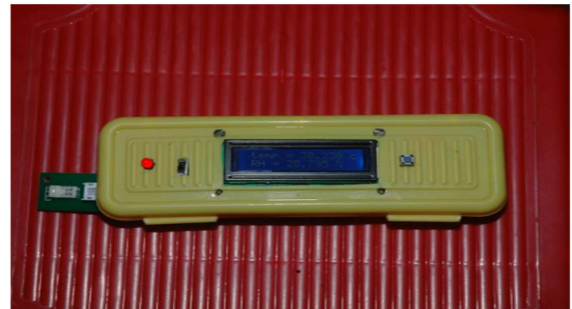
Fig. C1. Photograph of HSM 20G (humidity and temperature measurement sensor) interfaced with PIC 18F25K20 microcontroller
