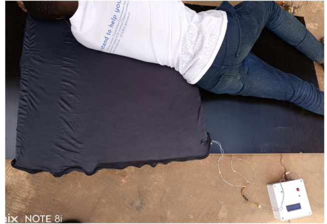
Figure 11. The successful testing and experimentation with the design and constructed low-cost pressure and temperature sensing mattress.
