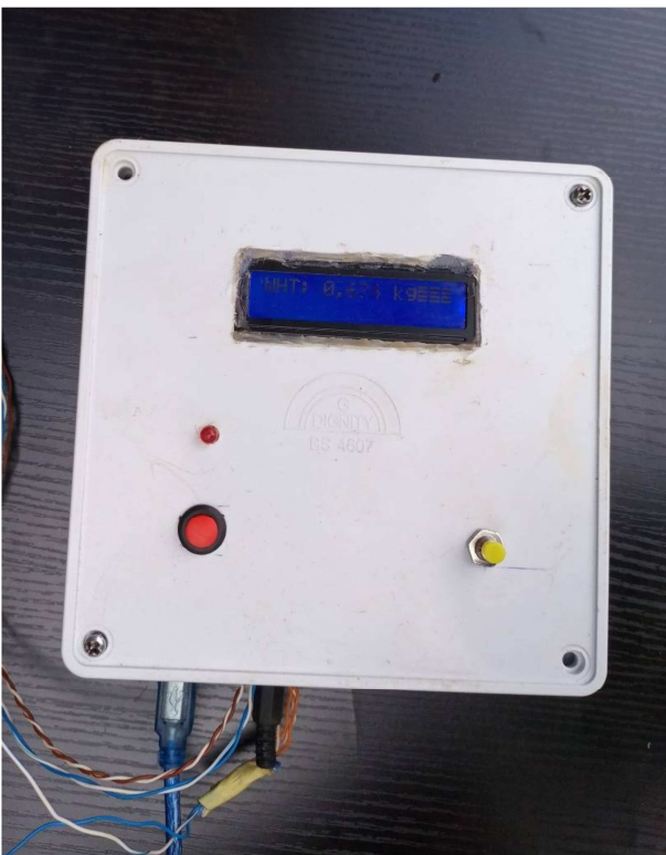
Figure 9. The complete control unit of the pressure and temperature sensing mattress.
