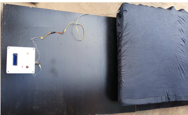
Figure 10. The complete experimental setup of low-cost pressure and temperature sensing mattress for testing and experimentation.
