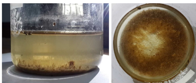
Figure 19. Coagulation process (Floc formation).
