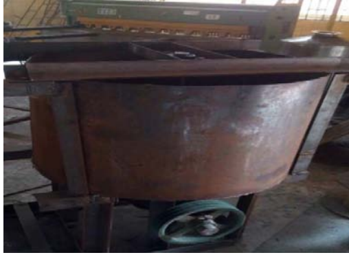
Figure 1. The Developed Concrete Mixer.
