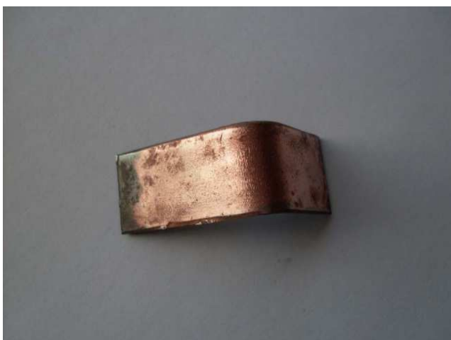
Figure 4. Sample coating after adhesion assessment by bending.
