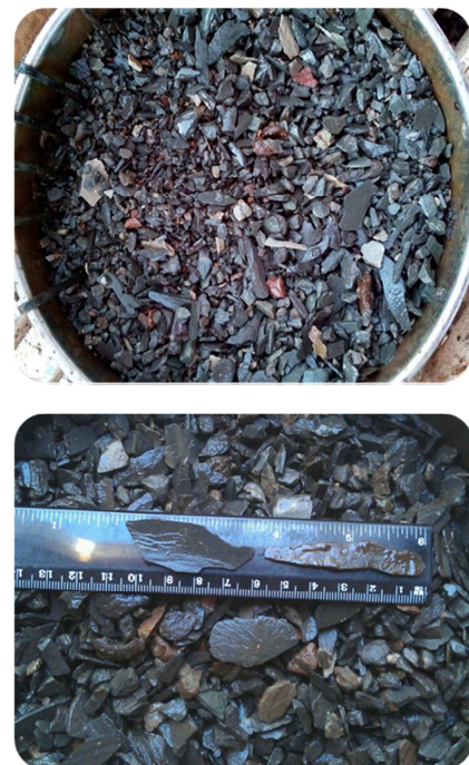
Figure 1. Cuttings falling from straight section of 8 1/4 "well section drilled earlier.
