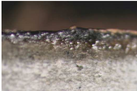
Figure 3. "Inner mud cake" formed by pf-chemseal in PIERRE II shale.
