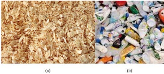
Figure 1. (a) Iroko sawdust, (b) high density polyethylene waste.
