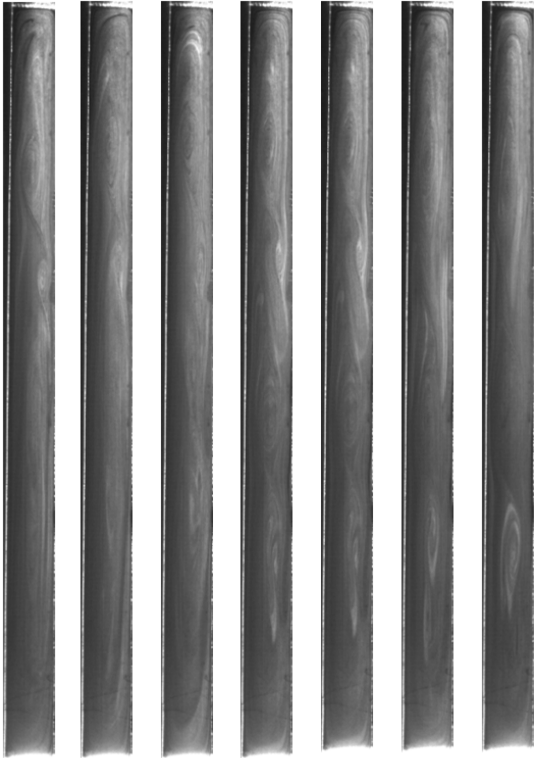
Figure 9. Flow growth inside the cavity for Ra=11772 ( \Delta T=23^\circ\text{C} ).
