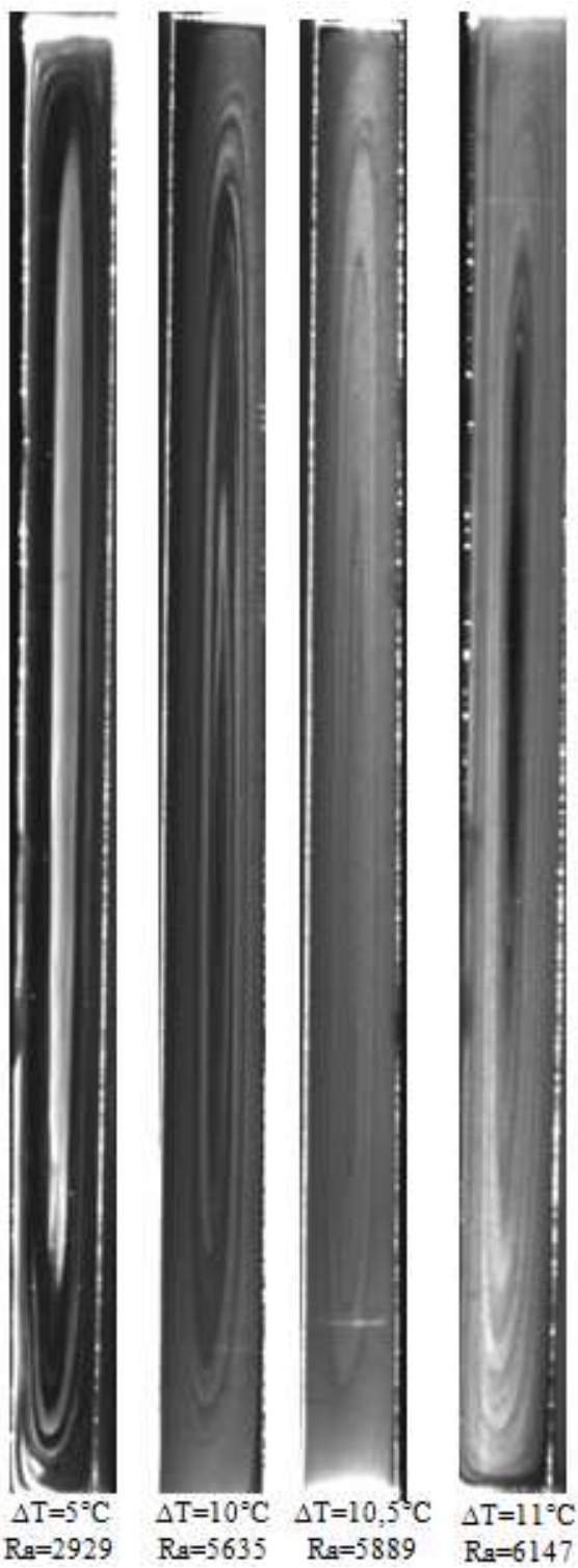
Figure 5. Flow patterns for different temperature difference and Rayleigh number.
