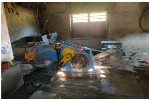
Figure 3. 29kW Microhydro powerplant existing in the village.
