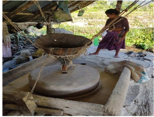
Figure 4. Water mill used for grinding mainly rice and maize.
