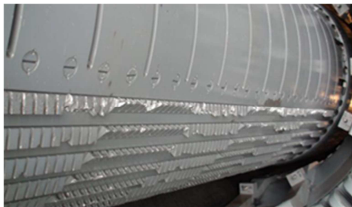
b) surface damages of bolts on rotor of the generator (around 200 pieces)
