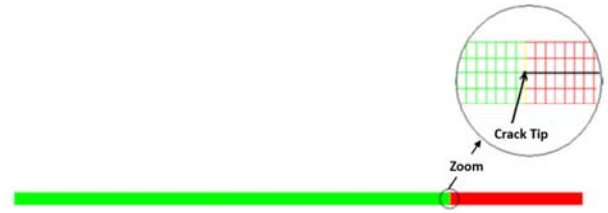
Figure 3. Interface element model in crack tip.
