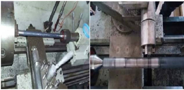
Figure 2. Burnishing operation.
