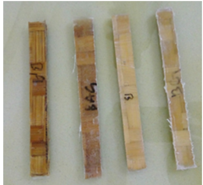
Figure 3. Test specimen for tensile and bending test.
