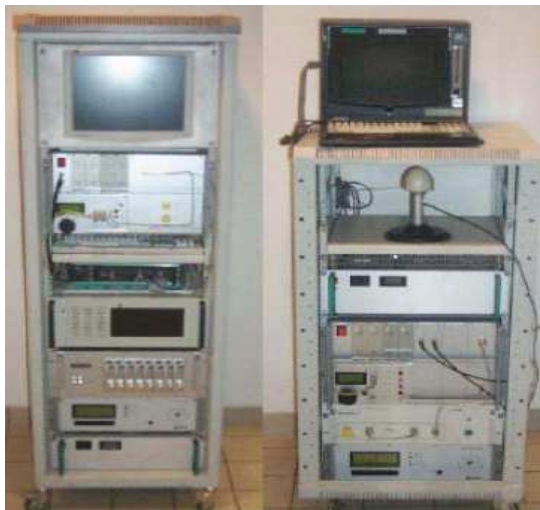
Figure 1. MIMO channel sounder: receiver and transmitter.
