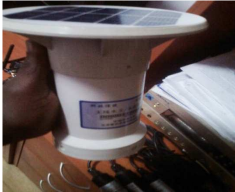
Figure 6. Solar Panel and final housing for Aquamesh.
