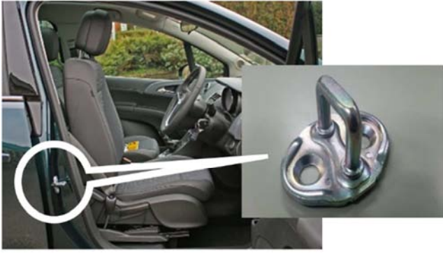
Figure 1. Automobile door striker.
