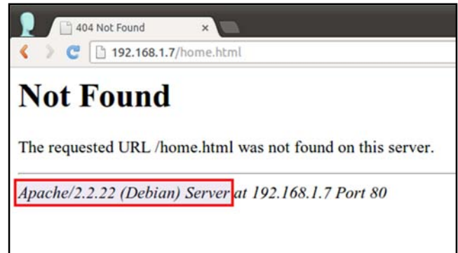
Figure 7. The error "Not Found" with revealed a web server signature.
