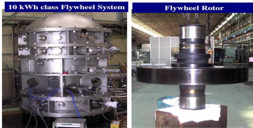
Fig. 18. Electricity storage system of flywheel type.
