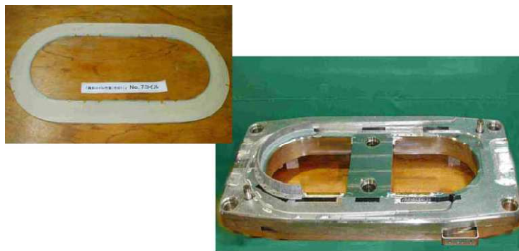
Fig. 19. Development of racetrack-shaped coil manufacturing technology.
