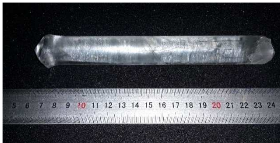
(b) The KDP crystal grown by the SR method
