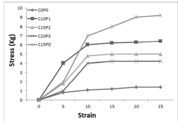
Figure 2. Tensile stress–strain curve for different Cellulose-PE composites.
