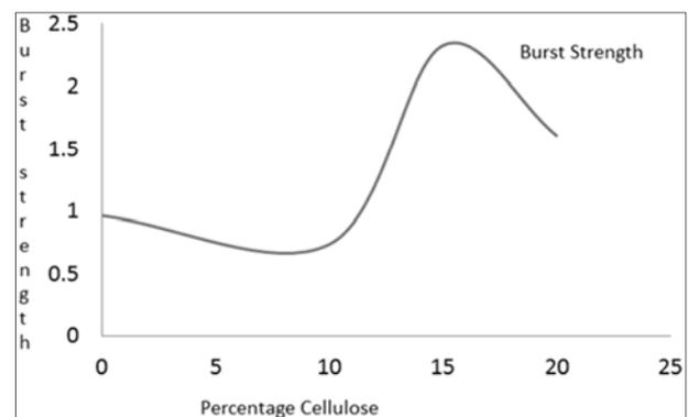
**Figure 6.** Burst Strength of Cellulose-PE composites.
