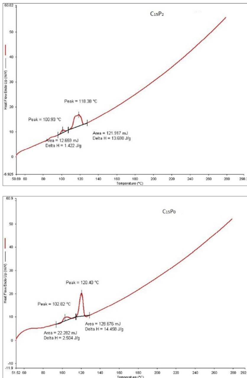
Figure 4. DSC curve of Cellulose-PE composites of pro-oxidant additives A) C<sub>15</sub>P<sub>2</sub> and B) C<sub>15</sub>P<sub>0</sub>.
