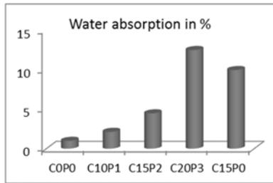
Figure 3. Water absorption percentage for Cellulose-PE composites.
