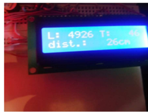
(b): LCD screen showing LDR analog data.
