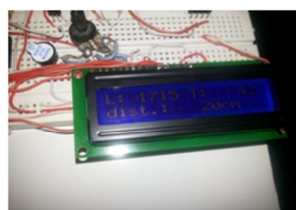
(b): LCD screen showing LDR analog data
