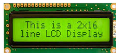
Figure 2. LCD screen 2 row×16 Column.
