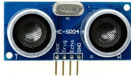
Figure 1. Ultrasonic sensor.
