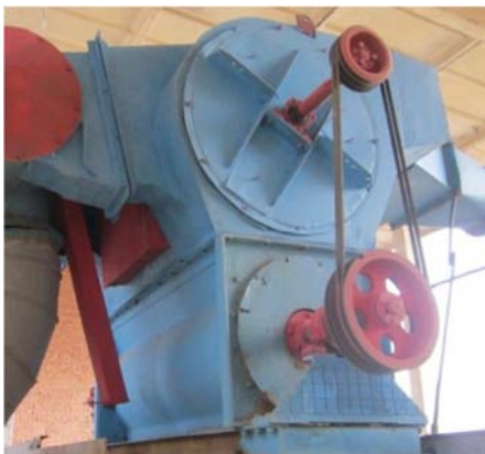
Figure 6. Cleaning separator of small impurities and heavy compounds in the cotton raw contain.
