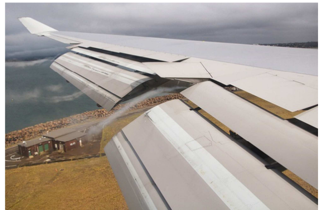
Figure 3. Flap of the wing.
