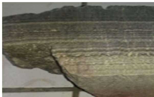
Figure 2. Fouling sample from the digestion step of phosphoric acid in wet phosphoric acid process.
