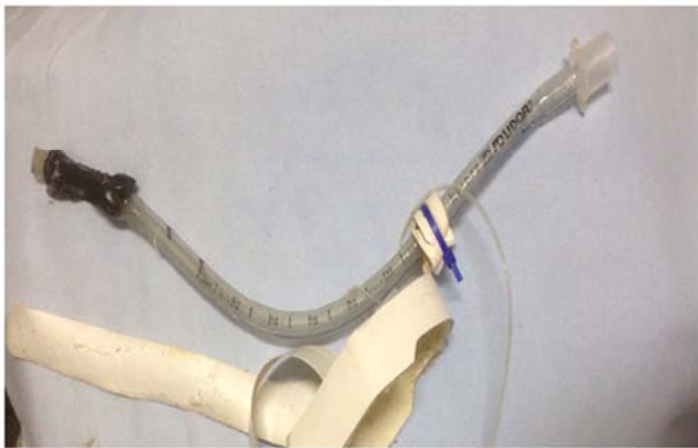
Figure 1. Endotracheal tube (SOLIDOR® 7.0) after combustion in the cuff area.
