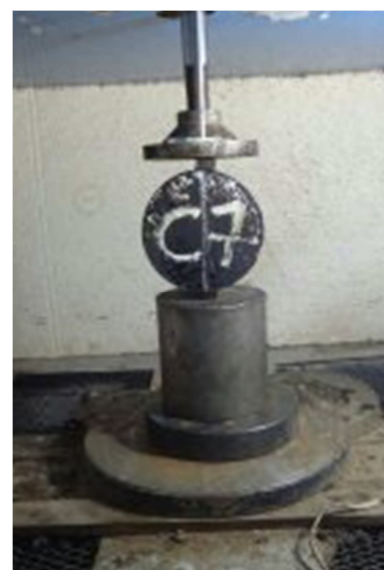
Fig. 2. ITS test setup.
