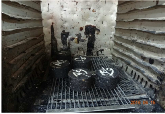
Fig. 3. Heating for crack healing.
