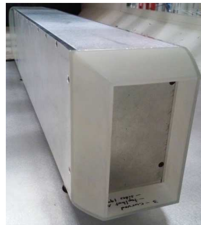
(c) Optimal design: curved, deflected base flaps.
