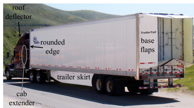
Figure 1. Example of straight trailer base flaps and other aerodynamic drag-reduction devices [2] (used with permission, ATDynamics/STEMCO).
