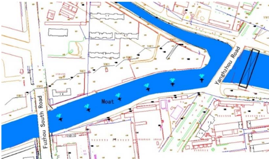
Figure 19. Layout of the purification section formed by the flap gate constructed at the end of the moat.
