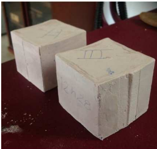
Figure 2. Test pieces obtained from the cubic molds.
