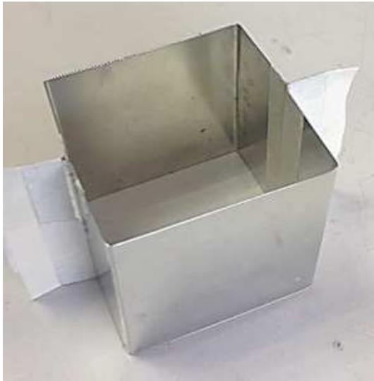
Figure 1. Metal foil mold used to obtain test pieces.
