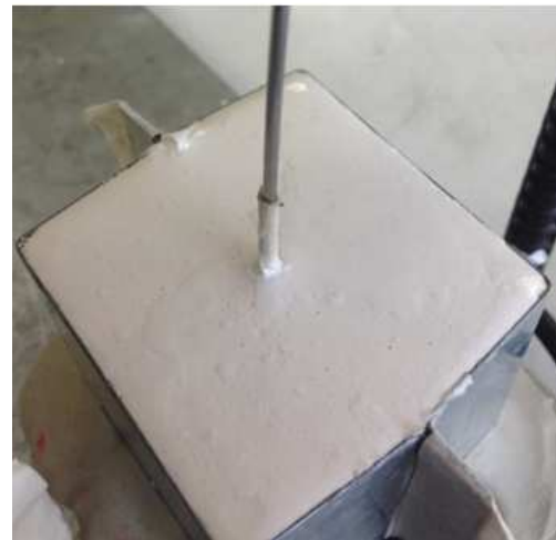
Figure 4. Position of the sensor for temperature measurement.
