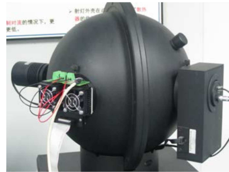
Figure 5. Electric power and optical power measurement employing Integrating sphere of TERALED.
