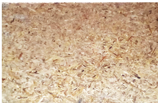
Figure 9. Particleboard of Sorghum bicolor stems.
