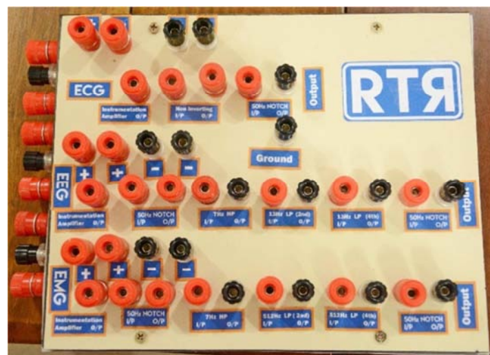
Figure 12. Designed prototype of RTR module. (a) Inner circuit blocks; (b) Side view. (c) Top view.
