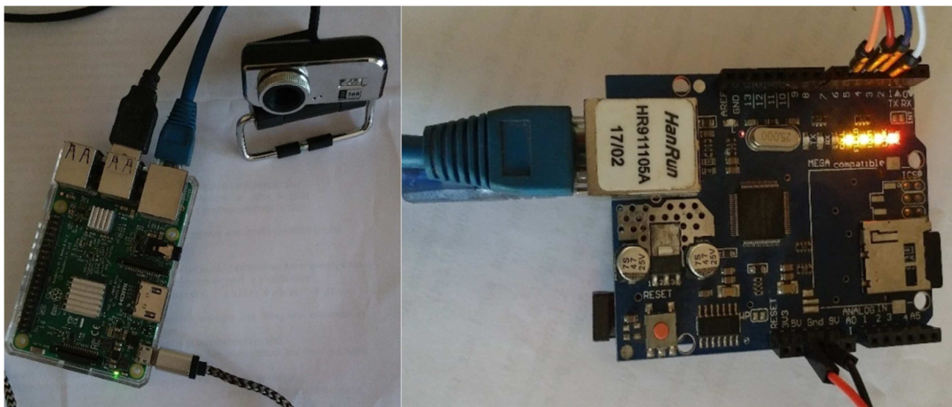
Figure 4. Real presentation of Raspberry Pi with USB camera and Arduino Uno with Ethernet Shield and SD card.
