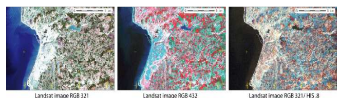
Figure 6. Digital image processing of LANDSAT ETM data merging different RGB band combinations with the panchromatic band
