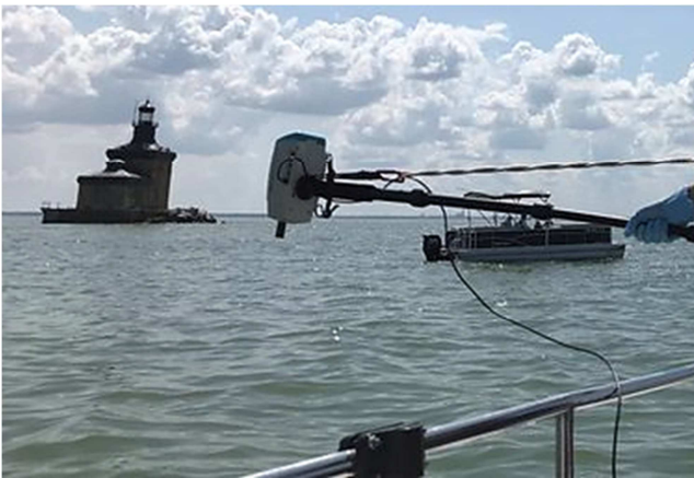
Figure 2. Actual Measurements Using Spectroradiometer Device on Lake Victoria.
