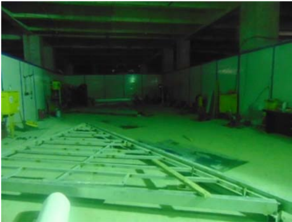
Figure 9. Making bed-jig from triangle frames.
