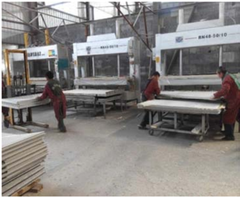
(c) Apply PU, place calcium silicate board
