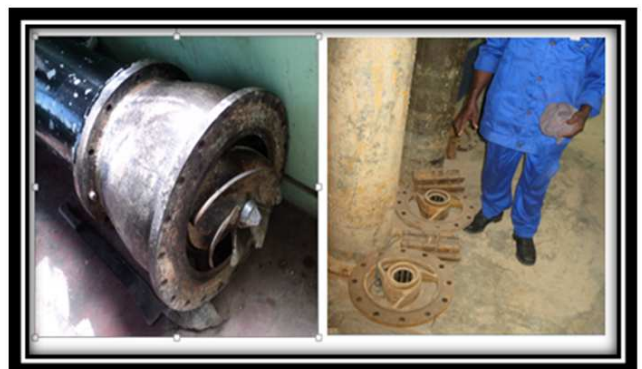
Figure 4. The Impacts of Illegal Mining on Pump Equipment.
