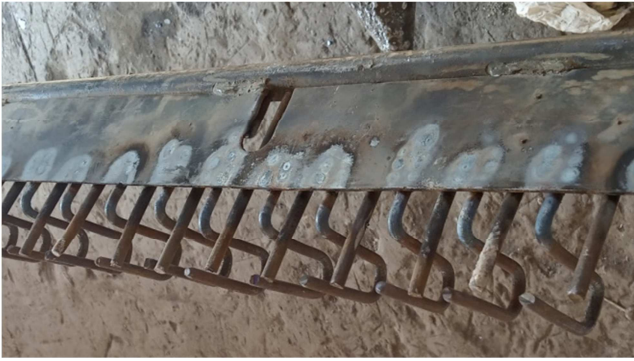
Figure 4. View of improved seed comb construction with additional slots.
