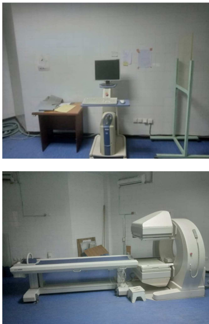
Figure 1. Gamma camera SPECT, double head brand MEDISO NUCLINE TM SPIRIT DH-V, with acquisition console on right (HOGIP).
