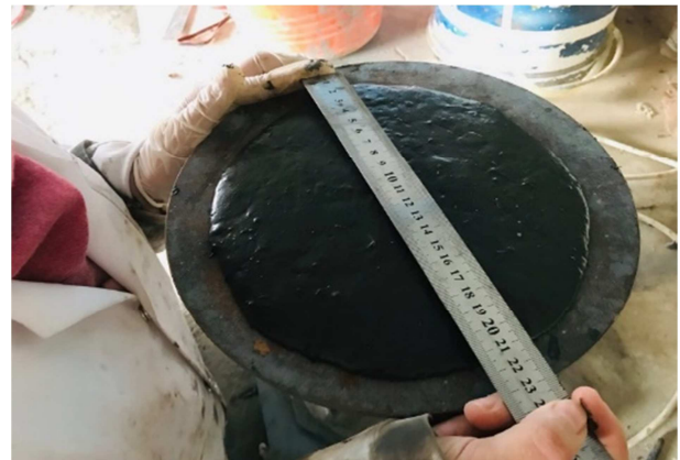
Figure 2. Flow Table test.
