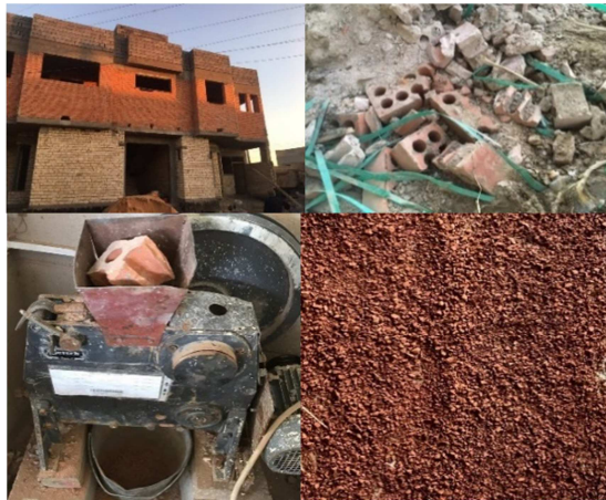
Figure 1. Crushed brick aggregate producing procedures.
