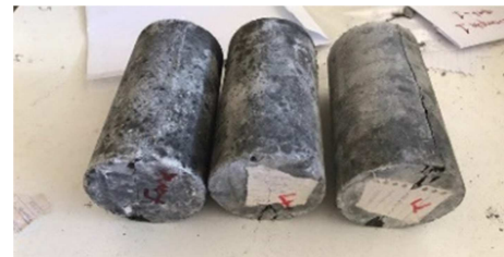
Figure 6. Mode of failure of splitting strength test.
