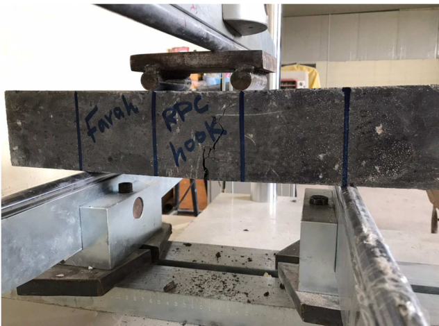
Figure 8. The failure mode of flexural strength test.
