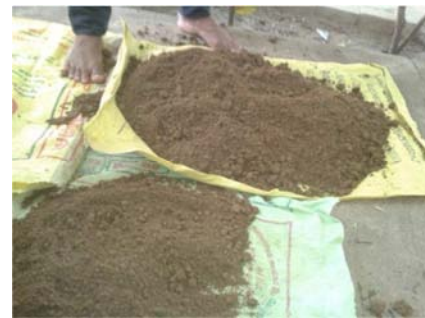
Figure 1. Verpavettuvan brick clay acquired on the depth of 1 to 1.5 m below the earth surface, which is located in Batticaloa District, Eastern Province of Sri Lanka.
