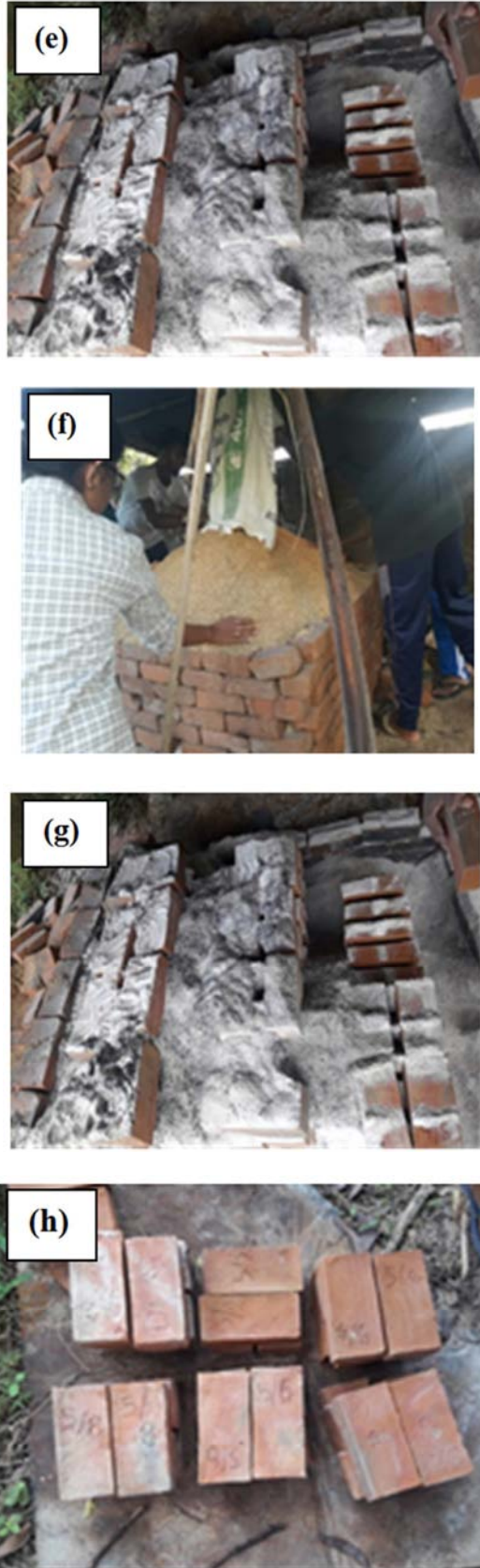
Figure 3. (a). Mixing clay and bamboo leaf ash, (b). Molding the mixture, (c). Green brick of dimension 185 mm x 85 mm x 65 mm, (d). Types of green bricks, (e), Conventional brick kiln, (f). Burning final stage and (g) burnt red clay-BLA bricks.
