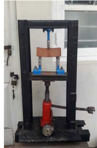
Figure 5. The brick has been ready to measure the point of force failure and the formation of crack indicates the force failure point.
