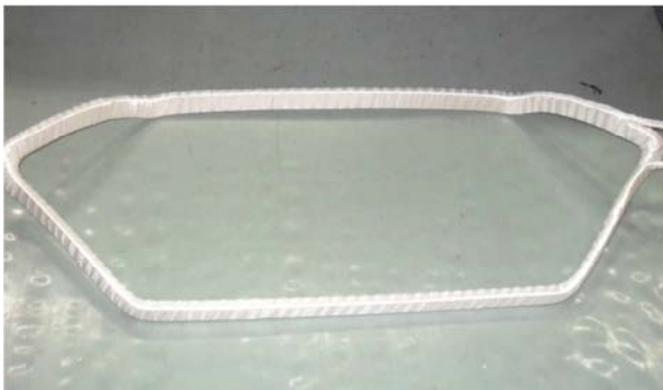
Figure 2. Winding without semiconductor layer.
