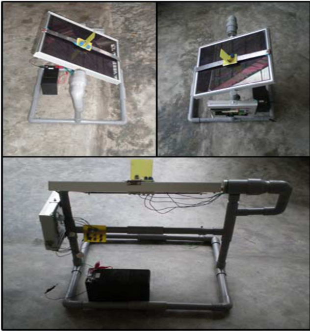
Figure 4. Constructed designed of a single axis sun tracking solar system modules [20]. 3.2.2. Dual (two) axis Active Solar Tracking System.
